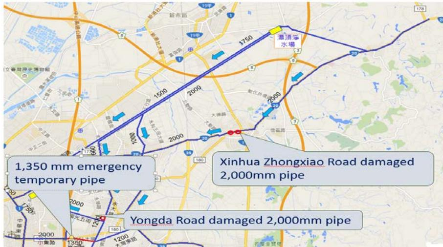
Fig.5 Location of damaged 2,000mm pipe and 1,350 mm temporary pipe
